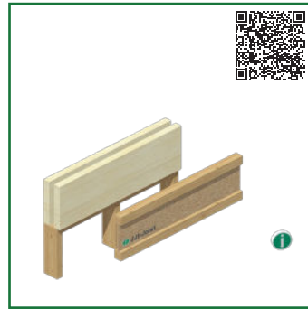
F33 - JJI-Joist parallel to party wall
