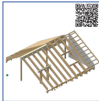
JJI-Joist pitched roof system
