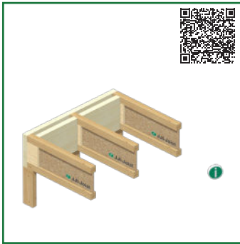
F32 - JJI-Joist bearing on party wall
