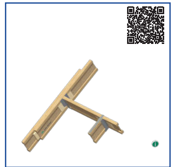
R8 - Opening in roof
