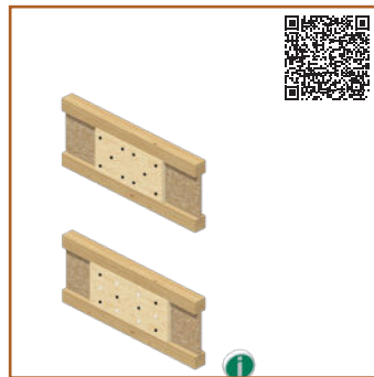
F21 - Filler and backer block nailing detail
